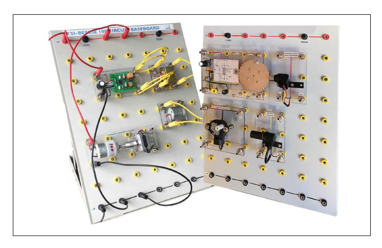
In addition to the basic automotive electrics/electronics and automotive sensors kits we also have special component set for EV/HEV technology.
