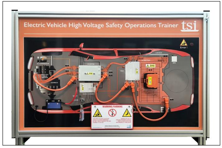
This mobile training stand has been specifically design to teach the principles of safe working on Electric Vehicles.
