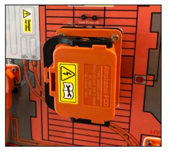
• The trainer incorporates real OEM EV components including cables and connectors as well as a Service Disconnect Plug
